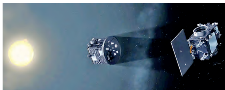
At regular intervals, one satellite will cast a shadow on the other, creating a makeshift total solar eclipse.
